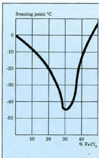
Figure 235. Freezing point of FeCl 3 solutions.
