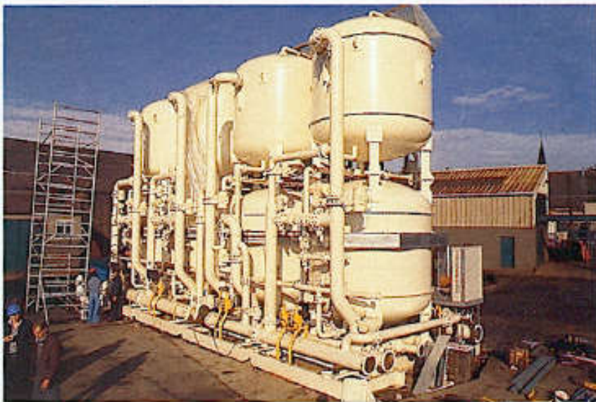
Figure 438. Sea water filtration skid for injection purposes. Shell installation at Fulmar (North Sea). Capacity: 1400 \text{ m}^3 \cdot \text{h}^{-1} .
