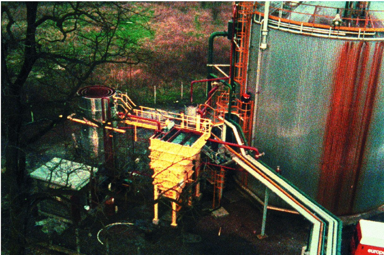
Figure 150. Aerobic reactor with a turbulent granular bed at the Beghin-Say sugar refinery in Thumeries in northern France.
