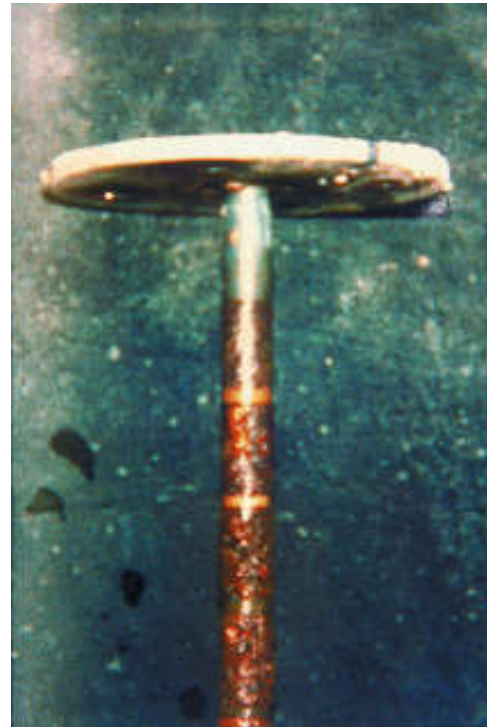
Figure 213. Coupon corroded by a softened water
