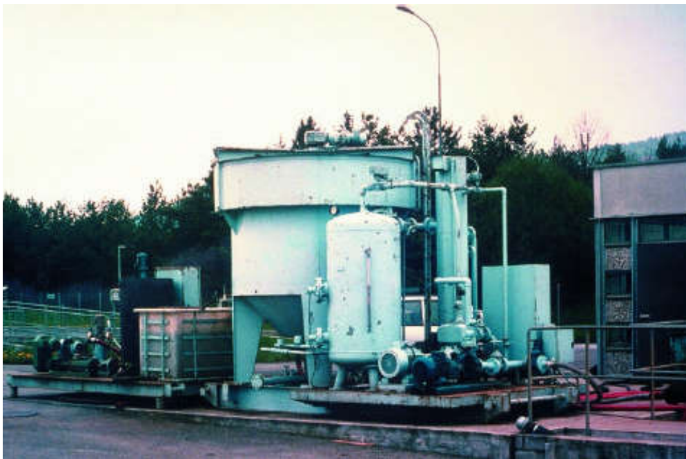
Figure 354. Mobile flotation unit. Flowrate: 10 \text{ m}^3 \cdot \text{h}^{-1} .
