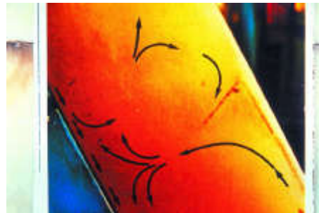
Figure 337. Sludge circulation between the plates of a Superpulsator.
