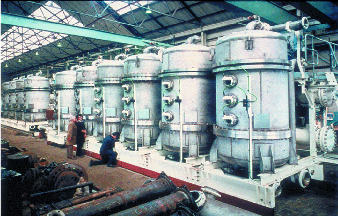
Figure 466. Shell Brent facility (North Sea). Flow rate: 1100 \text{ m}^3 \cdot \text{h}^{-1} . Candle filtration skid.
