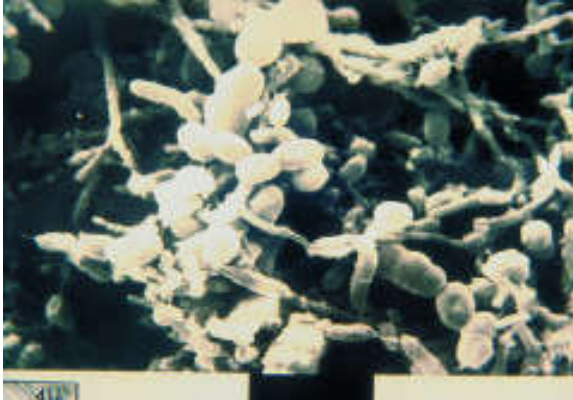
Figure 148. Enlarged view of an aerobic biological film on a granular support ( \times 1000 ).
