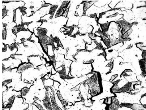
FIGURE 16.13 Hydrogen damage in a boiler tube; microstructure view.
