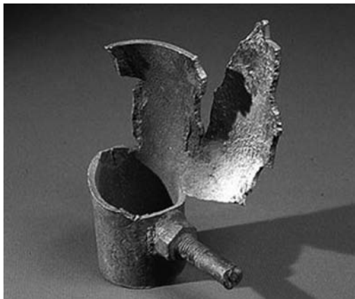
FIGURE 16.12 Hydrogen damage in a boiler tube.
