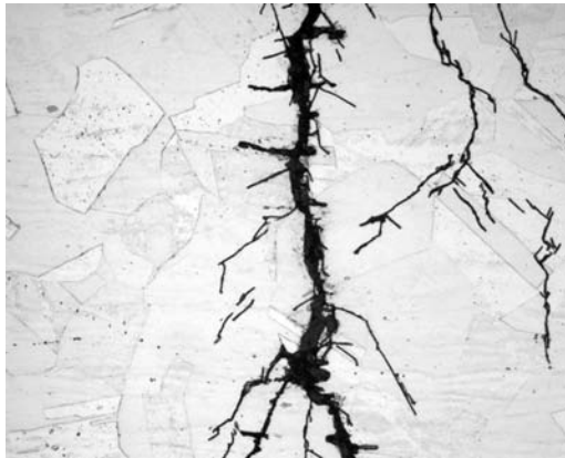
FIGURE 16.11 SCC of stainless steel due to chlorides; microstructure view.
