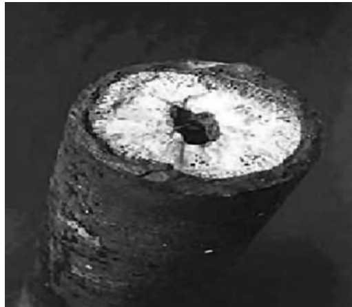
FIGURE 1.9 Barium sulfate scale deposit in an oil field pipeline.
