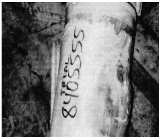
FIGURE 1.14 Fungus growth on an RO membrane.
