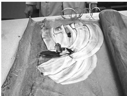
FIGURE 13.5 Fouled membrane. (From Kucera, J., Ultrapure Water , 22, 37, 2005. With permission.)
