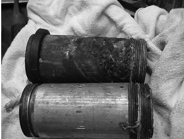
FIGURE 20.4 Scale built up on copper–silver electrodes in a poorly maintained flow cell.
