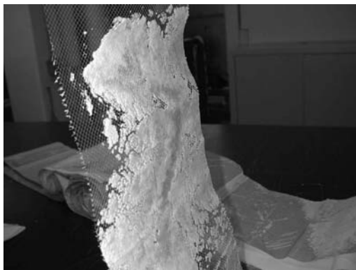
FIGURE 13.8 Scaled spiral wound membrane module feed spacer.
