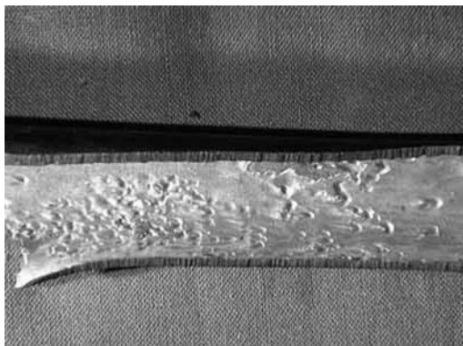
FIGURE 16.7 Erosion in brass. Note the horseshoe-shaped pits. Flow is from right to left.
